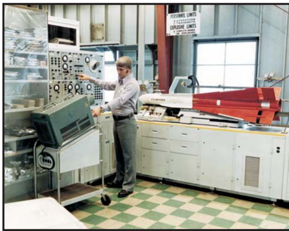
MATE (Micom Automated Test Equipment) tests circuit boards are used for the improved HAWK missile systems.
